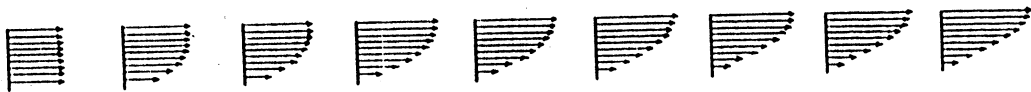
Figure 2 Velocity Vectors at Different Sections of a Straight Duct (Inlet Re = 153 , \Delta x = 0.24 m)
