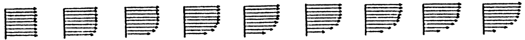
Figure 9 Velocity Vectors at Different Sections of a Straight Duct ( Uniform Inlet Re= 2750 , \Delta x= 0.24 m )
