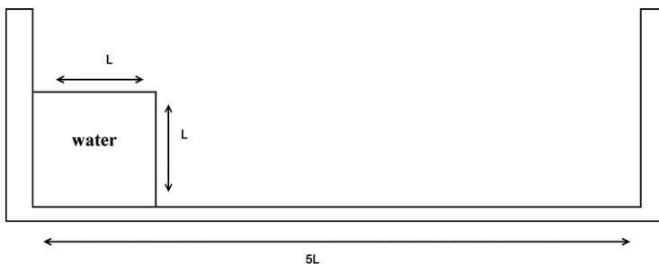
Figure 4. Schematic of the investigated dam-break problem.
