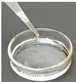
B. After 20 min in fume hood, solution is turned into clear gel
