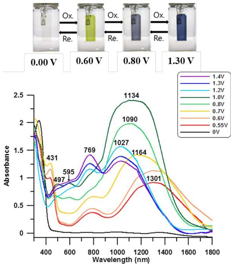
**Figure S21.** Spectroelectrochemistry of **PA2** at various applied potentials in 0.1 M TBAP/MeCN.
