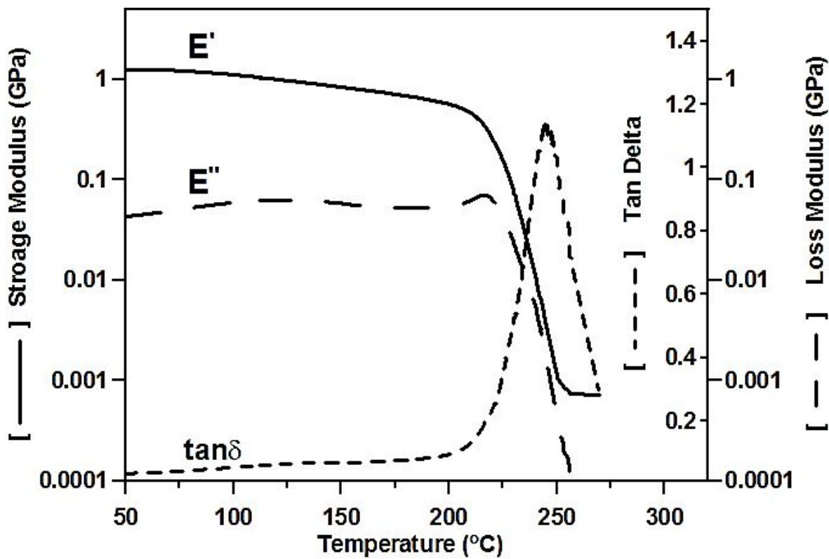
**Figure S16.** DMA curve of PA1 at heating rate 5°C/min.
