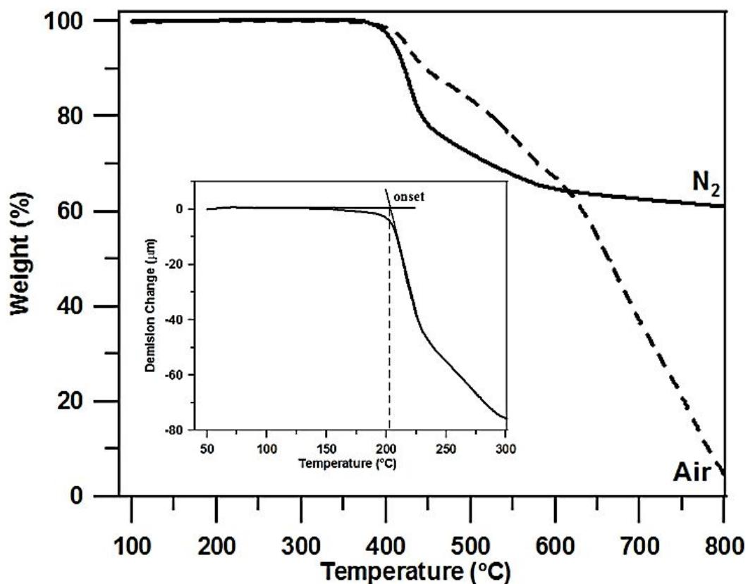
**Figure S14.** TMA and TGA curves of **PA1** at a heating rate of 10 °C/min and 20 °C/min.
