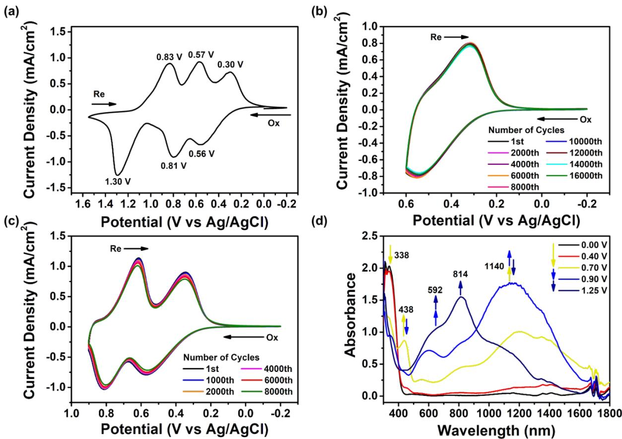
**Figure S19.** Cyclic voltammetric diagram of **PA1'** film (thickness:  $175 \pm 10 \text{ nm}$ ) at a scan rate of 50 mV/s (a) from -0.20 V to 1.55 V and its cyclic stabilities at (b) first oxidation stage (-0.20 V to 0.60 V) for 16,000 cycles and second oxidation stage (-0.20 V to 0.90 V) for 8,000 cycles in 0.1 M TBAP/MeCN. (d) Spectroelectrochemistry of **PA1'** (thickness:  $330 \pm 20 \text{ nm}$ ) at various applied potentials in 0.1 M TBAP/MeCN.
