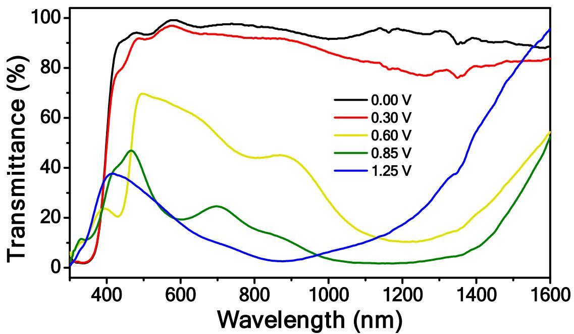
**Figure S22.** Optical change in transmittance of PA1 at various applied potentials in 0.1 M TBAP/MeCN.
