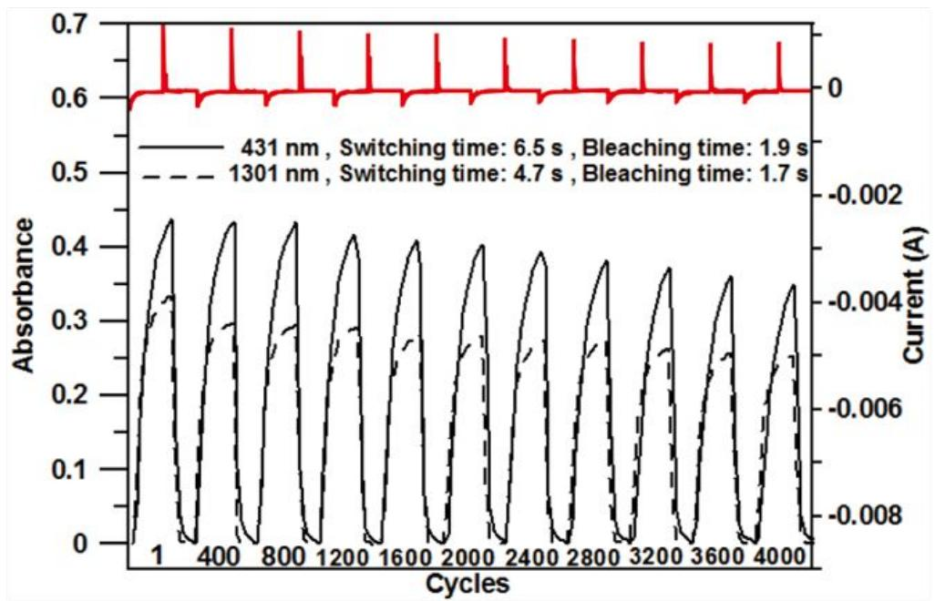
**Figure S23.** Potential step absorptometry and current consumption of **PA2** (in MeCN with 0.1M TBAP as the supporting electrolyte) by applying a potential step  $0.00\text{ V} \leftrightarrow 0.55\text{V}$ , and cycle time 20 s.
