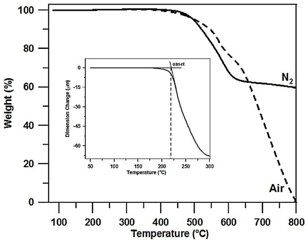
**Figure S15.** TMA and TGA curves of **PA2** at a heating rate of 10 °C/min and 20 °C/min.
