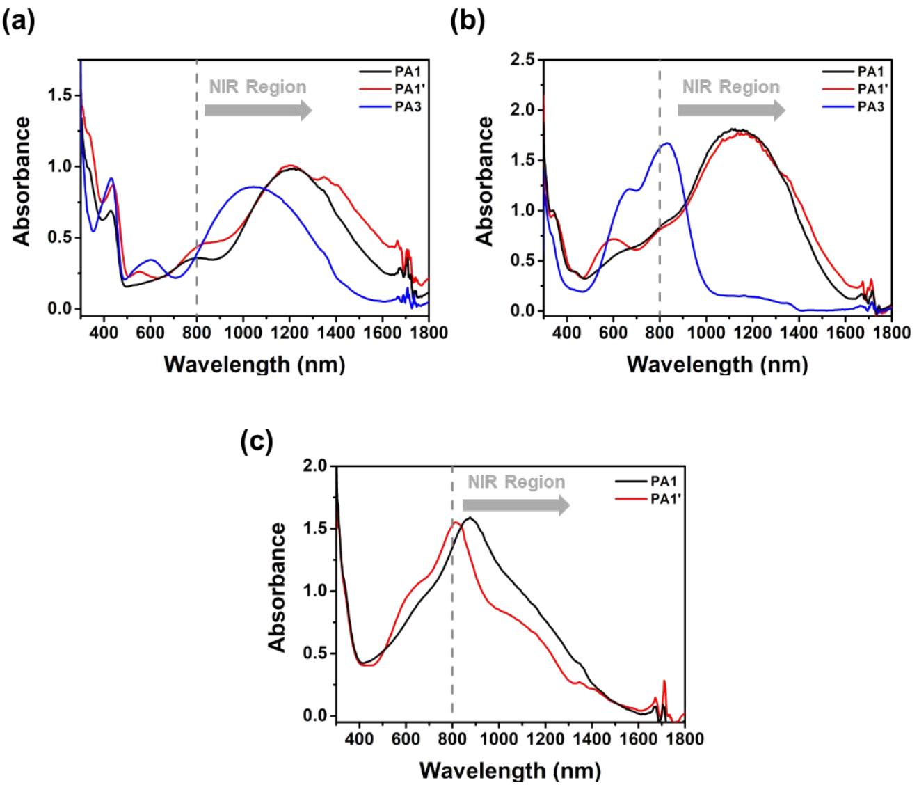
**Figure S24.** UV-vis-NIR absorption spectra of **PA1** (thickness:  $330 \pm 20$  nm), **PA1'** (thickness:  $330 \pm 20$  nm), and **PA3** (thickness:  $310 \pm 20$  nm) films at (a) first, (b) second, and (c) third (only **PA1** and **PA1'**) oxidation stage.
