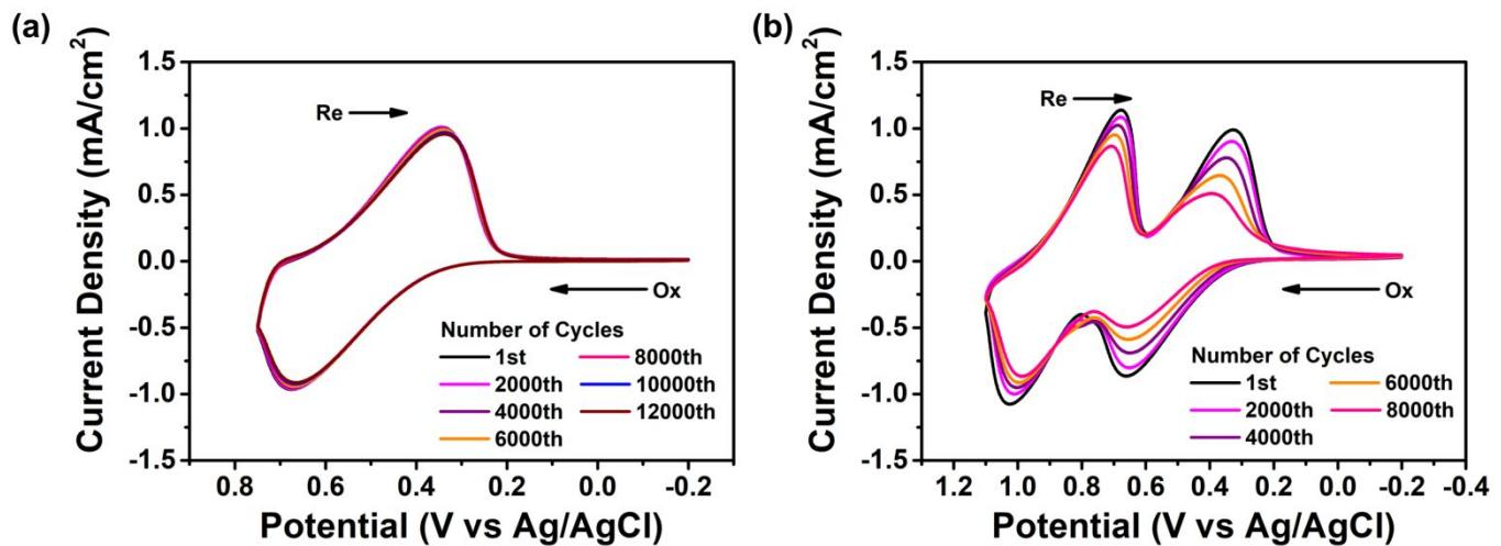
**Figure S20.** Cyclic stabilities of PA3 film (thickness:  $180 \pm 10 \text{ nm}$ ) at (b) first oxidation stage (-0.20 V to 0.75 V) for 12,000 cycles and (b) second oxidation stage (-0.20 V to 1.10 V) for 8,000 cycles in 0.1 M TBAP/MeCN.
