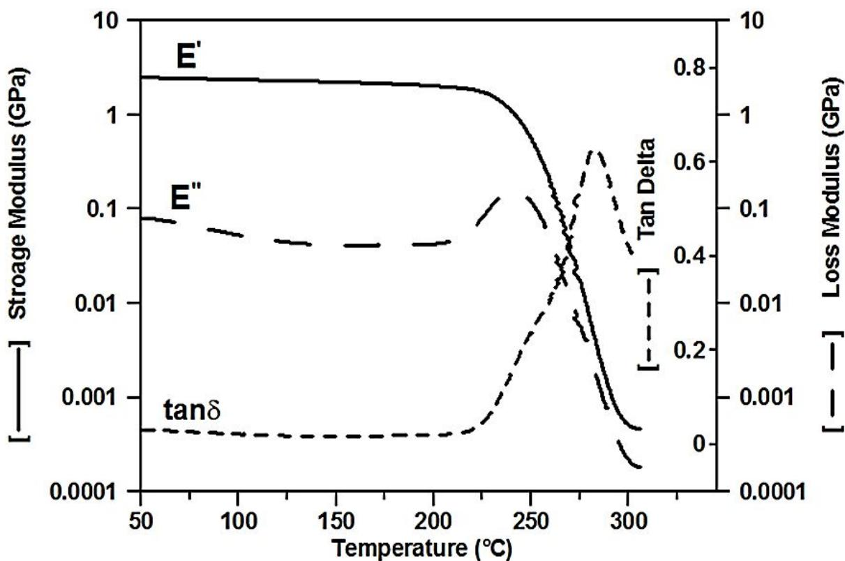
Figure S17. DMA curve of PA2 at heating rate 5°C/min.
