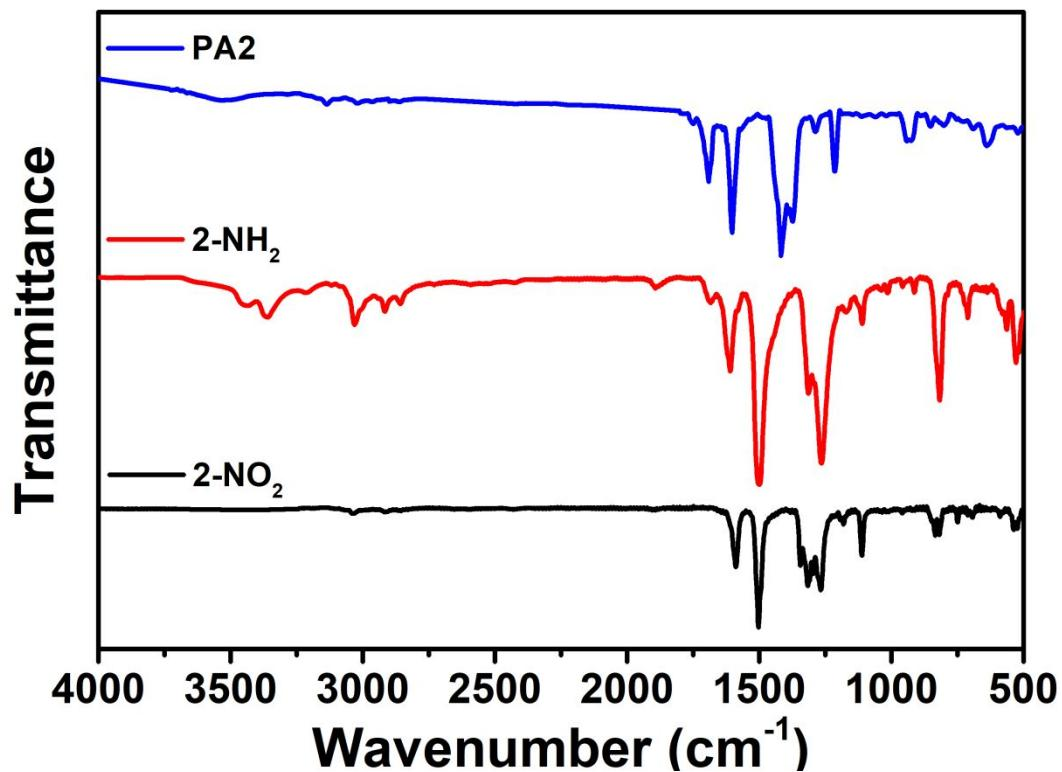
**Figure S2.** FT-IR spectra of 2-NO<sub>2</sub>, 2-NH<sub>2</sub>, and PA2.
