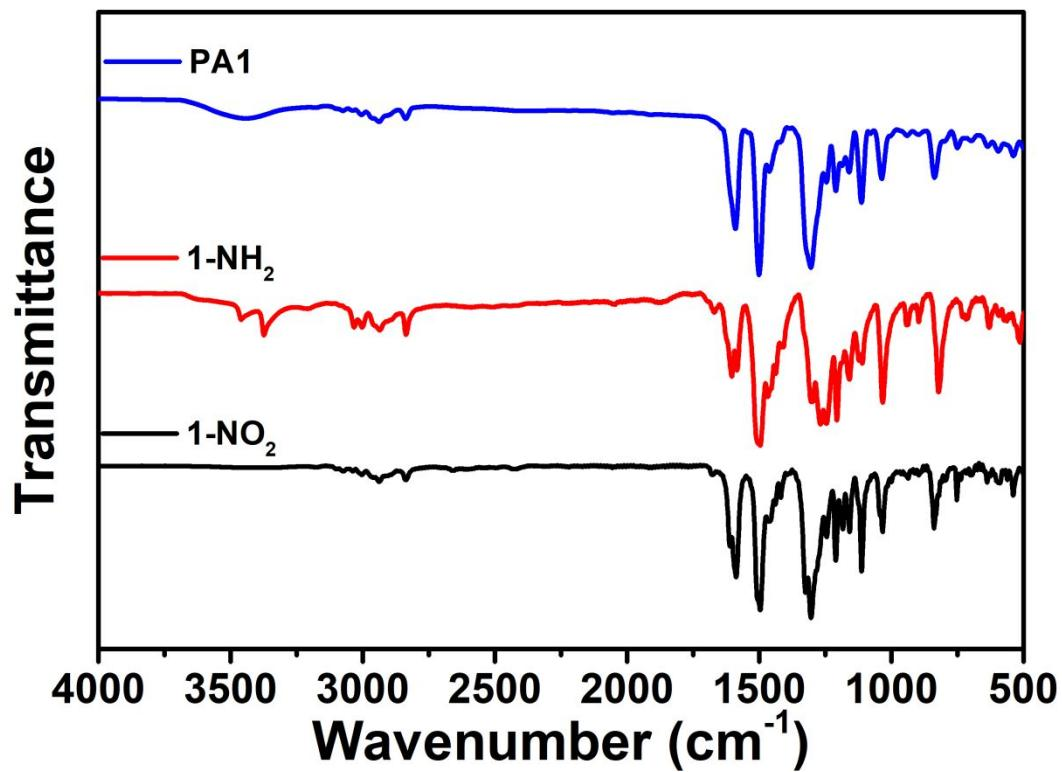
**Figure S1.** FT-IR spectra of **1-NO<sub>2</sub>**, **1-NH<sub>2</sub>**, and **PA1**.
