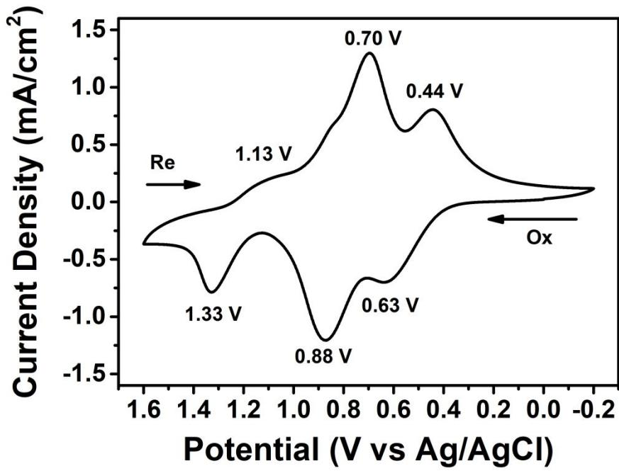
**Figure S18.** Cyclic voltammetric diagram of PA2 film (thickness:  $180 \pm 20$  nm) at a scan rate of 50 mV/s from -0.20 V to 1.55 V in 0.1 M TBAP/MeCN.
