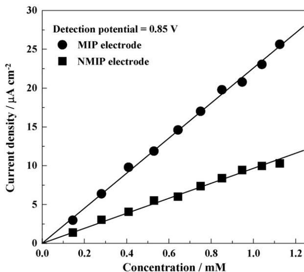
**Fig. 5.** Calibration curves of MIP (solid spheres) and NMIP (solid squares) electrodes with 0.6 wt% of the polymer in each case.
