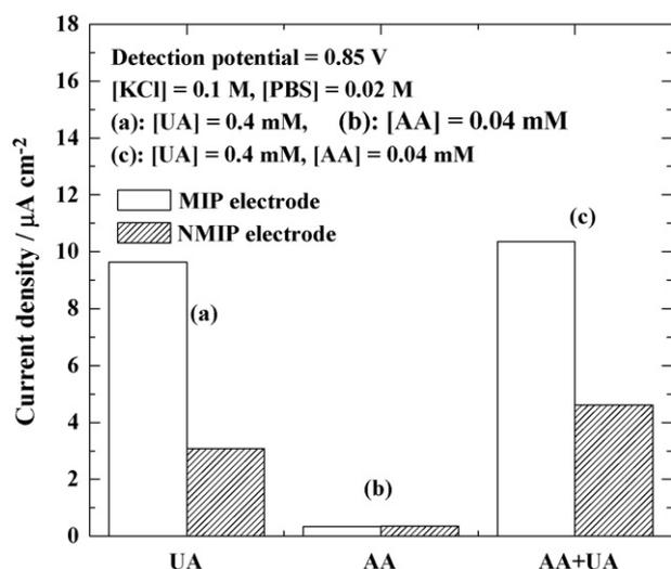
Fig. 8. Current density responses of the MIP and NMIP electrodes with 0.6 wt% of the polymer for (a) 0.4 mM of UA, (b) 0.04 mM of AA, and (c) 0.4 mM of UA + 0.04 mM of AA.
