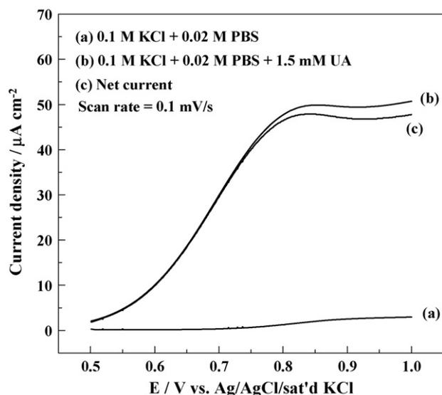
**Fig. 4.** Liner sweep voltammograms of MIP electrode in (a) 0.1 M KCl + 0.02 M PBS, and (b) 0.1 M KCl + 0.02 M PBS + 1.5 mM UA, at the scan rate of 0.1 V s<sup>-1</sup>. This figure also shows the net current (c).
