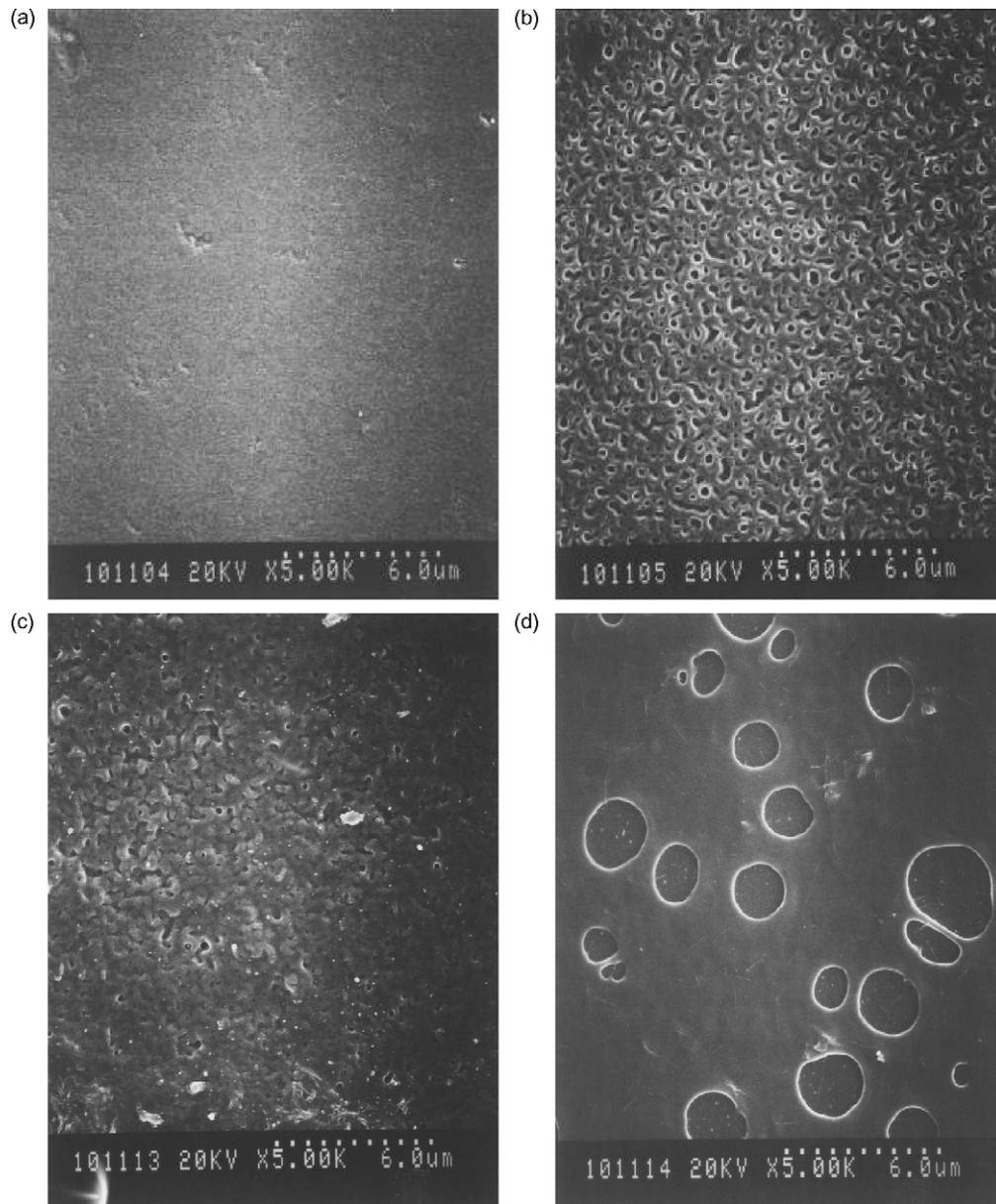
**Fig. 6.** SEM images of (a) NMIP electrode with 0.6 wt% of the polymer, (b) MIP electrode with 0.6 wt% of the polymer, (c) MIP electrode with 0.9 wt% of the polymer, and (d) MIP electrode with 0.3 wt% of the polymer.
