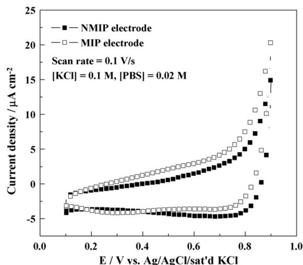
**Fig. 3.** Charge capacities of MIP electrode (□) and NMIP electrode (■) after the extraction of UA, both CVs being obtained in 0.1 M KCl + 0.02 M PBS (pH 7.4) at the scan rate of  $0.1 \text{ V s}^{-1}$ .
