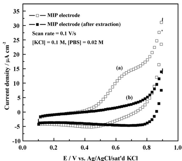
**Fig. 2.** CVs of the MIP electrode with 0.6 wt% of the polymer, in 0.1 M KCl + 0.02 M PBS (pH 7.4) at the scan rate of  $0.1 \text{ V s}^{-1}$ : (□) before extraction of UA and (■) after its extraction.
