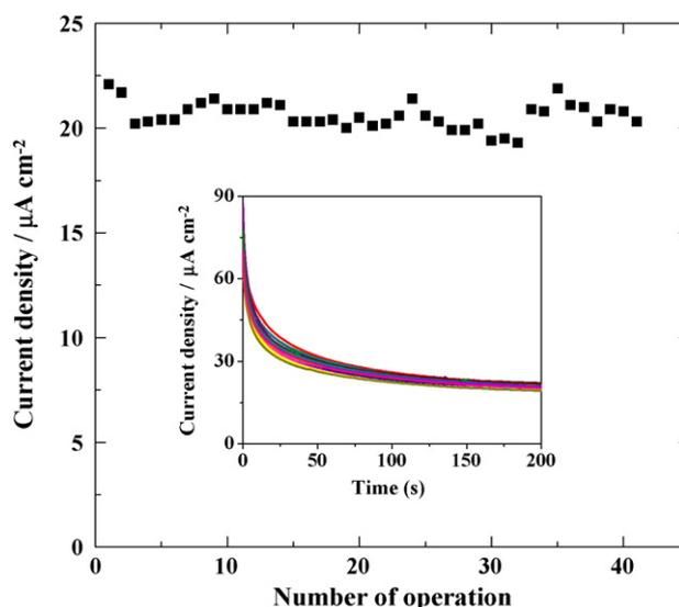
Fig. 9. Reusability of the MIP electrode with 0.6 wt% of the polymer for 40 operations.
