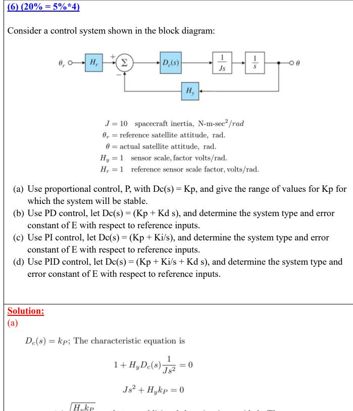
or  $s = \pm j \sqrt{\frac{H_y k_P}{J}}$  so that no additional damping is provided. The system cannot be made stable with proportional control alone.
