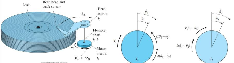
Model (Equations of Motion: Rotational motion)
