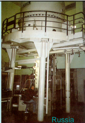
3 MV Ultra-High Voltage Electron Microscope
