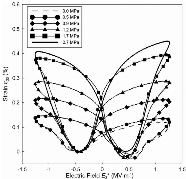
FIG. 2. Measured strain vs electric field hysteresis curves for (001)-oriented BaTiO<sub>3</sub> single crystal at various constant compressive stresses.
