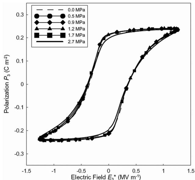
FIG. 1. Measured polarization vs electric field hysteresis curves for (001)-oriented BaTiO<sub>3</sub> single crystal at various constant compressive stresses.
