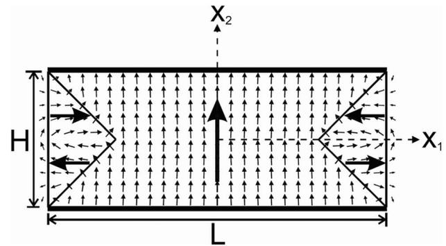
FIG. 3. Compatible domain pattern in a  $5 \times 2 \text{ mm}^2$  BaTiO<sub>3</sub> single crystal [the heavy arrows denote the polarizations, while the small arrows denote the directions of electric displacement vector ( $\mathbf{D}$ )].
