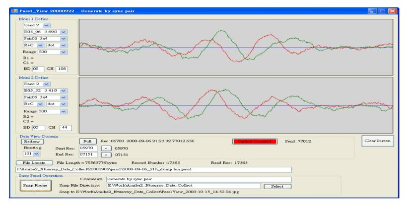
Fringes of two adjacent channels of 275Mhz Verify the system temperature =  $90^{\circ}$ K +  $40^{\circ}$ K
