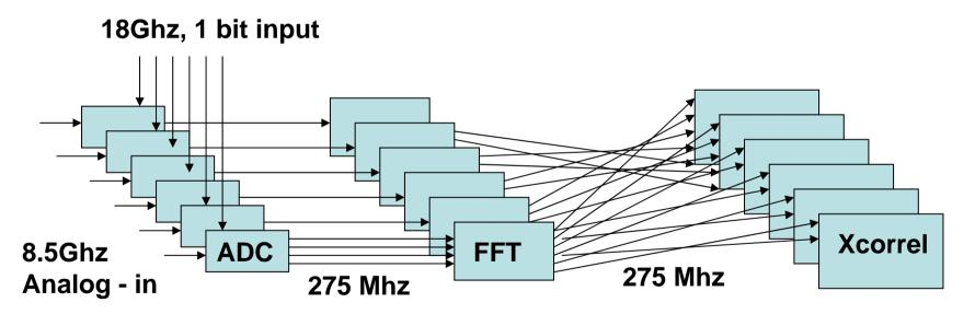
Digital Correlator for One Band of 8.7Ghz NTU Array has 4 bands of a total 35Ghz bandwidth
