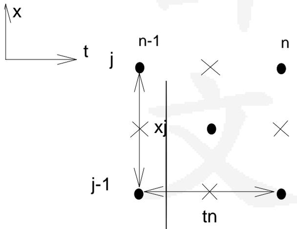
$$\left\{ \begin{aligned} \frac{u_j^n - u_{j-1}^n}{\Delta x_j} = v_{j-\frac{1}{2}}^n = \frac{1}{2} (v_j^n + v_{j-1}^n) \end{aligned} \right. \quad (7-33)$$
