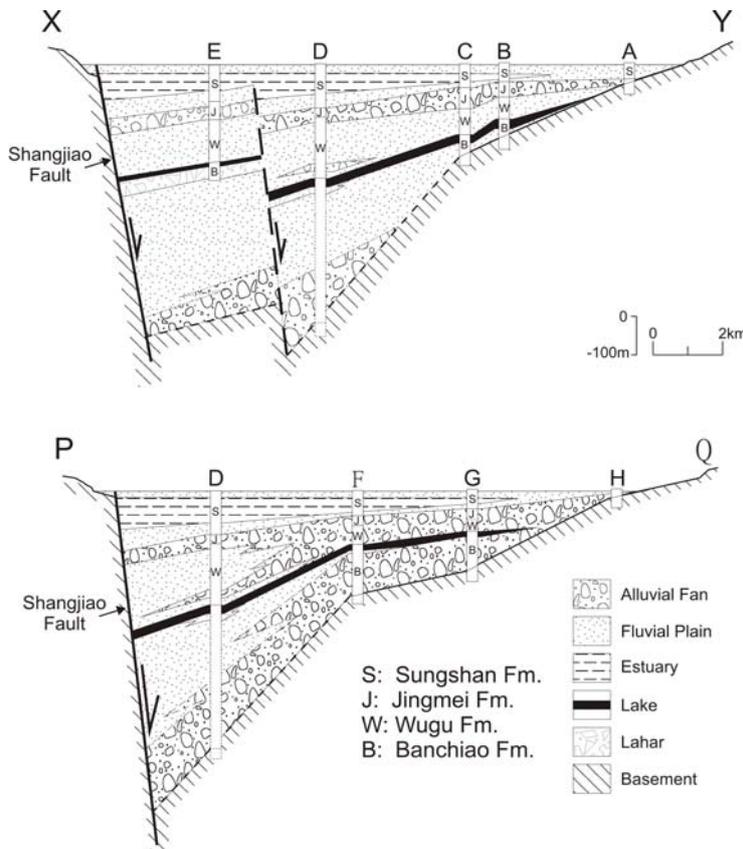
Figure 4. Facies characteristics and basin configuration. Note the inferred normal fault in section X-Y and the exaggerated thickness of deep-lake deposits. Facies characteristics of the lower part of Borehole D are based on unpublished data of Central Geological Survey. Borehole locations shown in Figure 3; stratigraphy in Figure 9.
