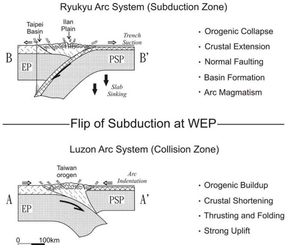
Figure 6. Geodynamic configuration. Upper panel shows that the Taipei Basin sits on the frontal part of the collapsing orogen with arc magmatism in the north. Before the subduction polarity flipped, the orogen underlying the Basin was part of the rising orogen similar to that of the active collision zone shown in the lower panel. EP: Eurasian plate; PSP: Philippine Sea plate. Modified from Teng and Lee (1996); locations shown in Figure 5.
