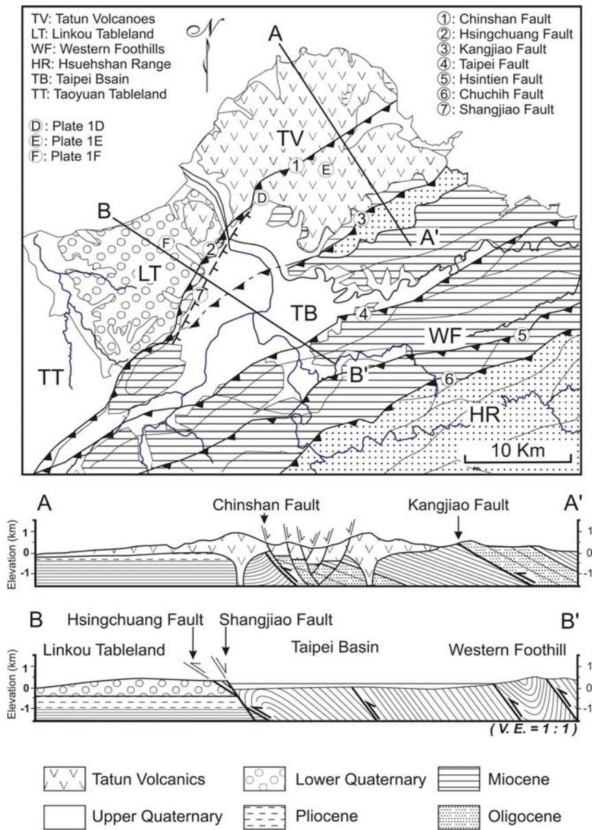
Figure 2. Geological setting of the Taipei Basin. Note that both Hsingchuang and Chinshan Faults are overprinted by extensional structures and a rift basin underlies the Tatun volcanics. Top map modified from Ho (1986); Section A-A' from Chu *et al.* (1998).
