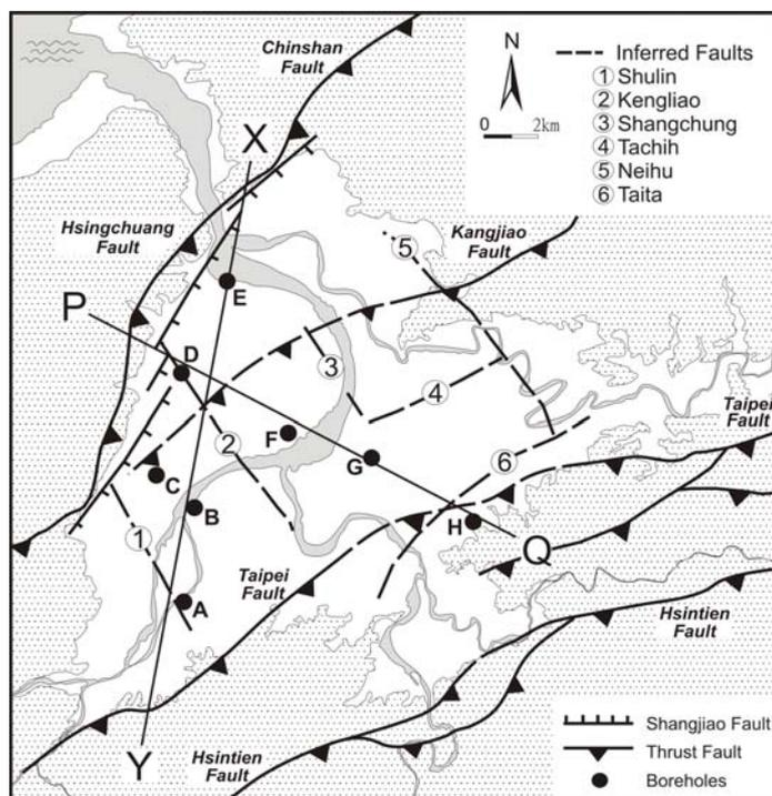
Figure 10. Structural features. Sections X-Y and P-Q shown in Figure 4. Modified from Ho (1974, 1983); Inferred faults from Wang Lee *et al.* (1978).
