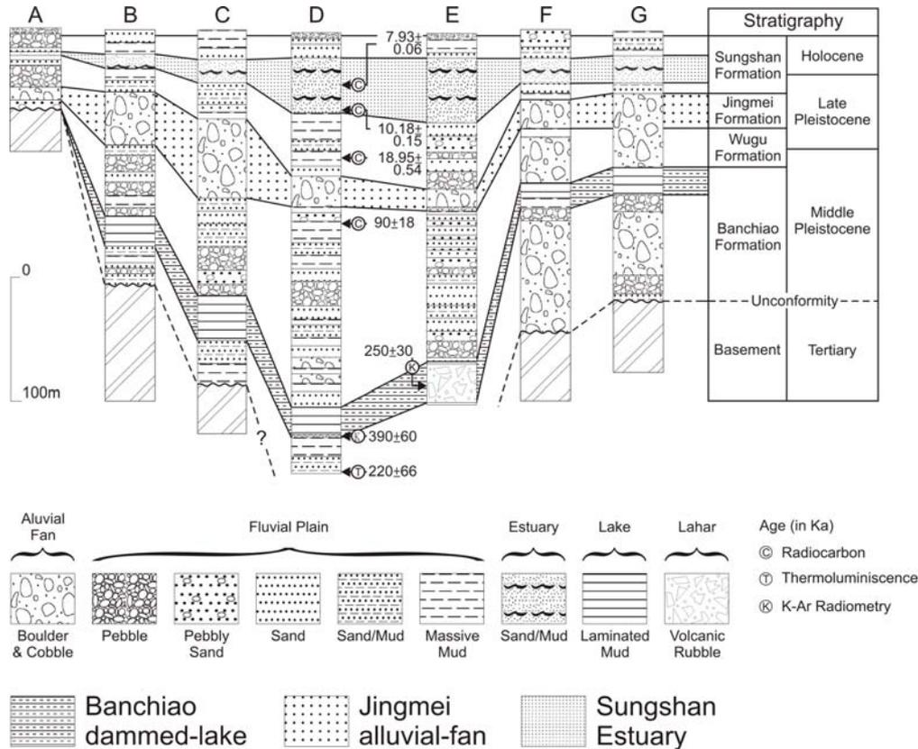
Figure 9. Borehole stratigraphy and depositional events. Location and symbols of boreholes shown in Figure 4. Modified from Teng *et al.* (1998); Radiocarbon dates from Liu *et al.* (1994); K- Ar dates from Chen *et al.* (1995) and Tsao (1997); Thermoluminescence dates from Wei *et al.* (1998)
