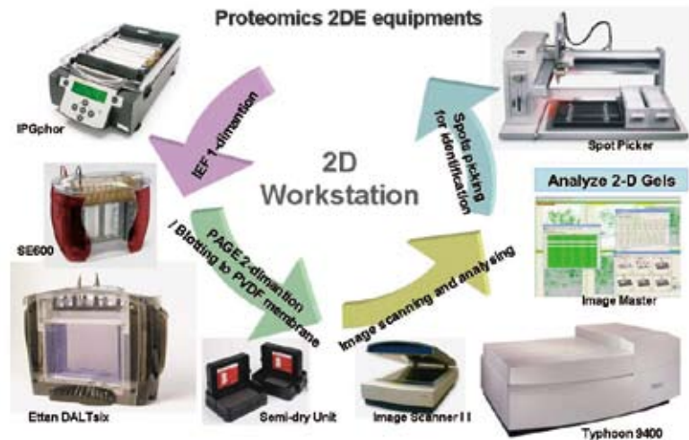
The Proteomics and Protein Function Core Laboratory's workflow for two-dimensional electrophoresis analysis
