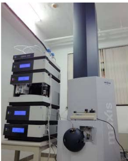
Fig. 1: The Metabolomics Core provides a quadrupole-time of flight Mass Spectrometer (MaXis from Bruker) coupled with a UPLC system from Dionex.
