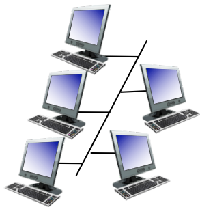
shared wire (e.g., cabled Ethernet)
