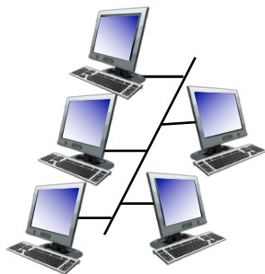
shared wire (e.g., cabled Ethernet)
