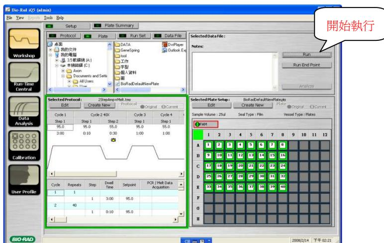
會自動跳到選擇 well factor 種類的視窗，點選“Collect Well Factors from Experimental Plate”
