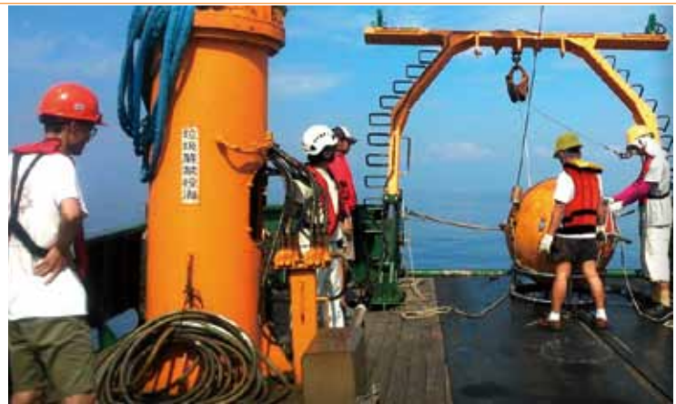
▲ Prof. Ming-Huei Chang (left) supervises the deployment of an ADCP mounted in the orange buoy (right) aboard the R/V Ocean Researcher III.
