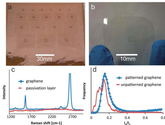
Fig. 2 (a) Patterns deposited by ink-jet printing on copper foil, (b) patterned graphene film after transfer to plastic substrate, (c) Raman spectra of graphene and passivation areas, (d) histograms of  $I_D/I_G$  ratio for graphene obtained on patterned substrate and pristine Cu foil.
