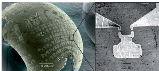
Fig. 5 False-color SEM image of lithographically patterned graphene transferred onto a 3 mm glass torus, (inset) magnification of feature with 5  $\mu\text{m}$  gap feature.
