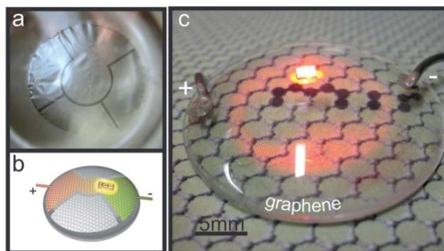
Fig. 4 Transfer of patterned graphene onto complex shaped objects. (a) Photograph of patterned graphene membrane during transfer, (b) schematic of graphene electrode structure, (c) photograph of patterned graphene electrodes on a lens supplying current to a LED.
