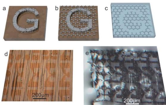
Fig. 1 (a–c) Representation of the procedure that results in patterned graphene (a) deposition of a passivation layer, (b) area-selective growth of graphene, (c) after removal of growth substrate (d) optical micrograph of copper foil after deposition of  $\text{Al}_2\text{O}_3$ -passivated patterns, (e) darkfield micrograph of resulting patterned graphene after Cu-removal (sample is floating on water during transfer, supported by a polymer membrane).
