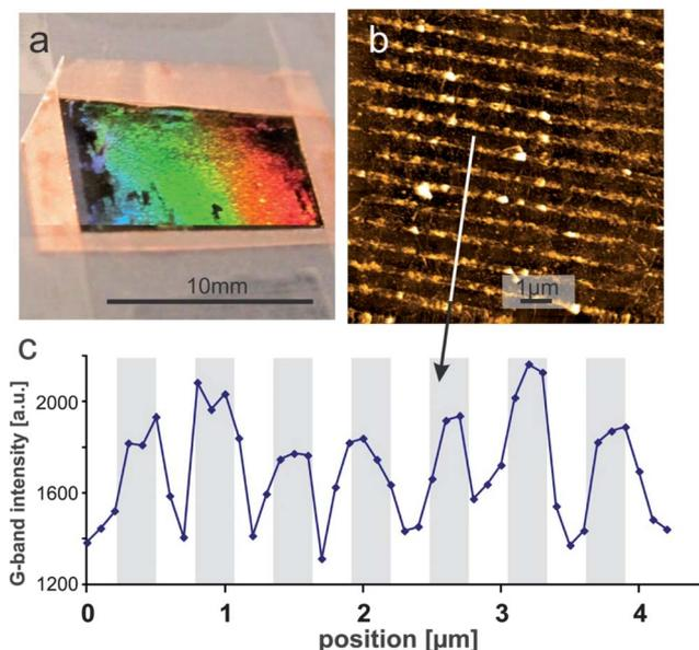
Fig. 3 (a) Photograph of copper foil patterned by microcontact printing deposition of a passivation layer, (b) AFM image of the resulting parallel  $\text{Al}_2\text{O}_3$  lines with a 700 nm period after growth and transfer (c) variation of G-band intensity across graphene stripes.
