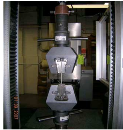
FIG. 4—The experimental set up for the tensile test of the latex membrane.
