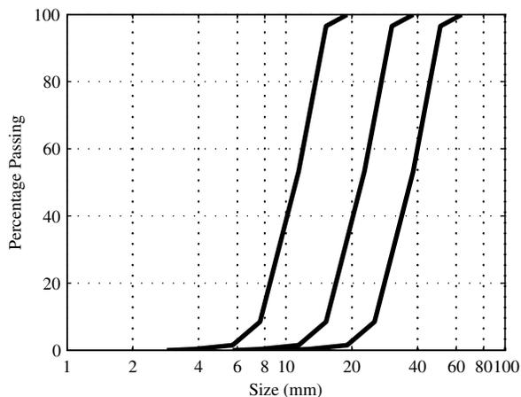
**Fig. 1.** Grain-size distributions of prototype and model gradations
