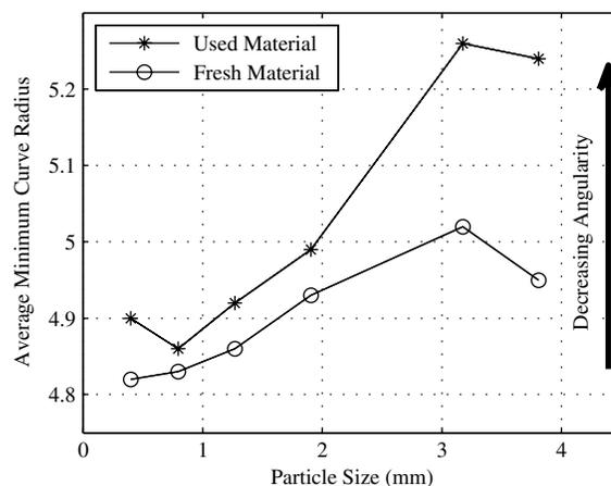
Fig. 9. Minimum inscribed curve radii of fresh and used particles
