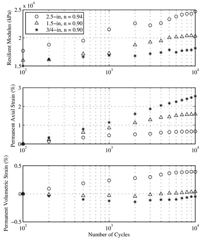
**Fig. 7.**  $n = 0.90$  resilient modulus, permanent axial strain, and permanent volumetric strain comparison
