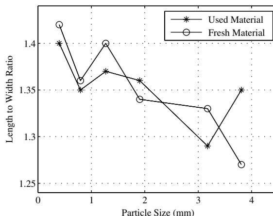
Fig. 8. Length to width ratios of fresh and used particles
