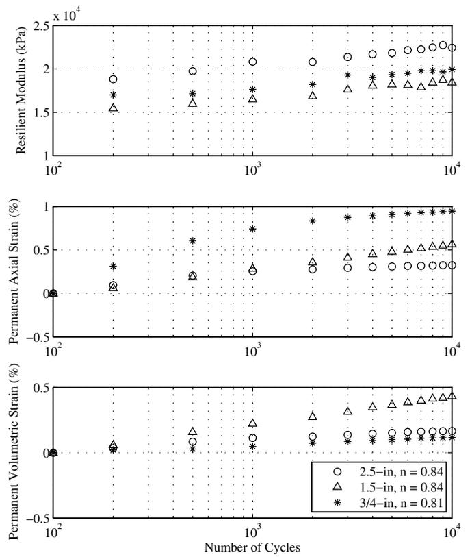
**Fig. 6.**  $n = 0.84$  resilient modulus, permanent axial strain, and permanent volumetric strain comparison
