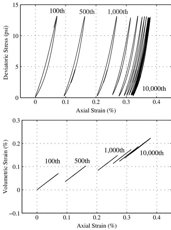
**Fig. 4.** Typical cyclic stress-strain response
