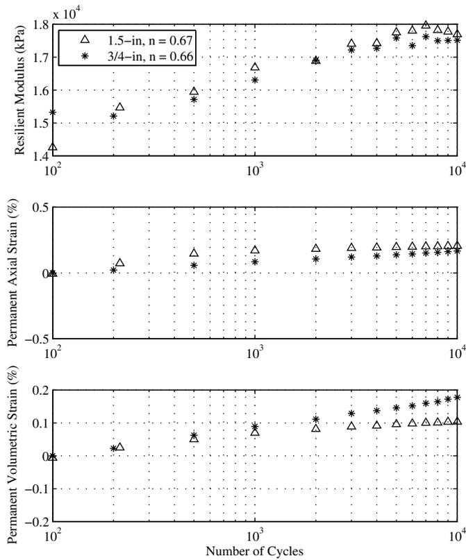
**Fig. 5.**  $n = 0.67$  resilient modulus, permanent axial strain, and permanent volumetric strain comparison
