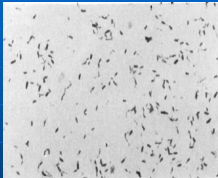
Rice-grain polyaniline particles using a graft copolymer stabilizer based on poly(ethylene oxide).
