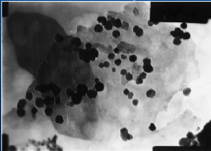
TEM micrograph of PANI/ \text{Fe}_3\text{O}_4 composite particles
