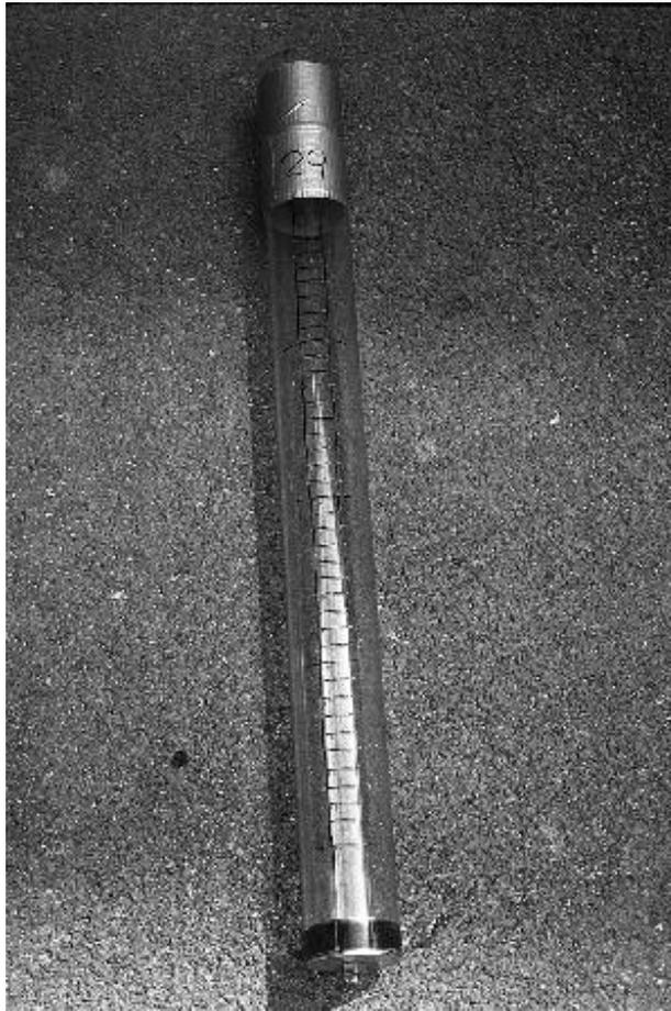
**Figure 4.4** The root observation tube (minirhizotron) used in this study.
