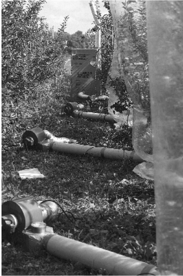
Figure 3.2 Photograph of the pipes, blowers, buffer tank, and canopy gas-exchange chambers on test trees at the experimental site in Geneva, N.Y.
