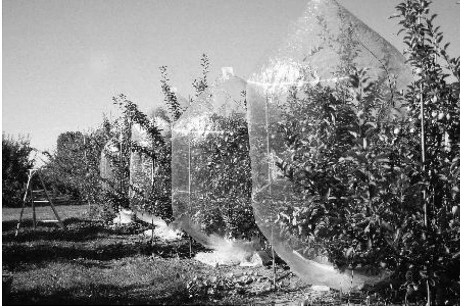
**Figure 3.1** Photograph of the open-flow "balloon" type gas-exchange chambers on test trees at the experimental site in Geneva, N.Y.
