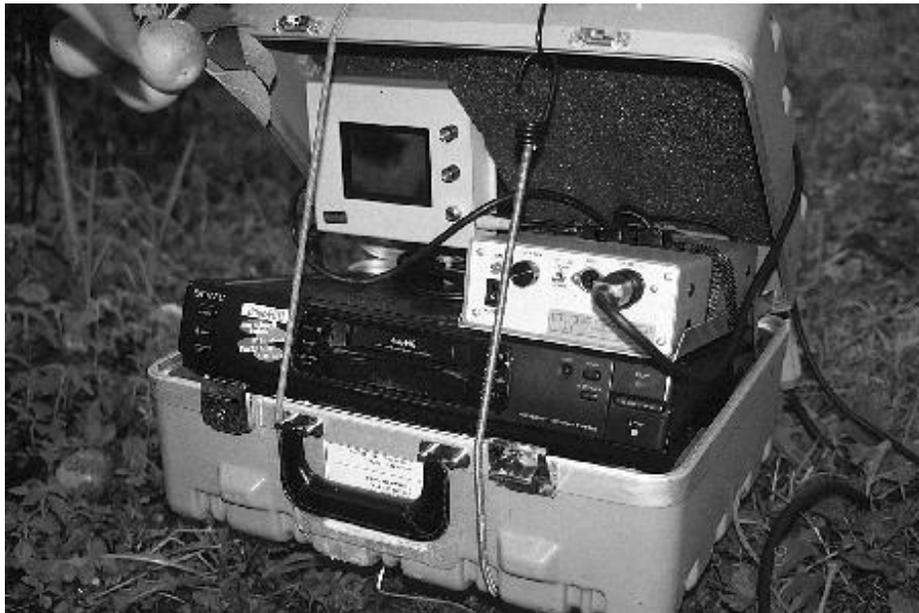
**Figure 4.1** The controller, monitor, and video cassette recorder (VCR) of the minirhizotron camera-VCR system (BTC-2, Bartz Technology, Santa Barbara, Calif.).
