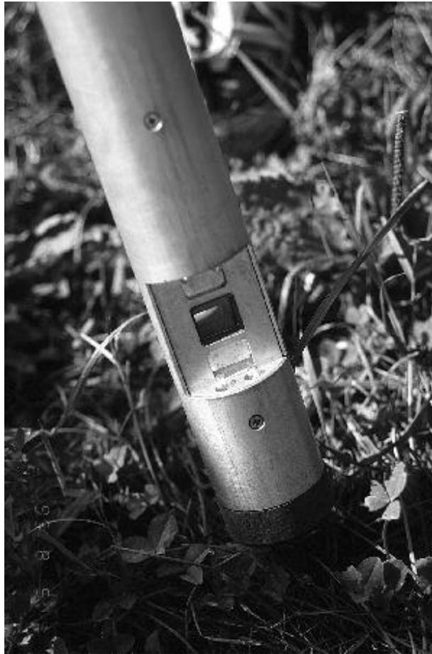
**Figure 4.2** The camera head module of the minirhizotron camera-VCR system (BTC-2, Bartz Technology, Santa Barbara, Calif.).
