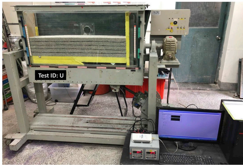
Fig. 3. The sandbox and test setup: (a) illustration; (b) panorama.
