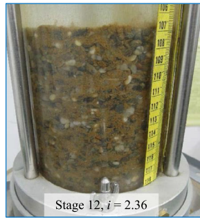
Fig. 12. Test results of R-0.3-6: (a) i-v curve, (b) and (c) at hydraulic failure, (d) at the next applied hydraulic head increment after i_{cr, failure} .
