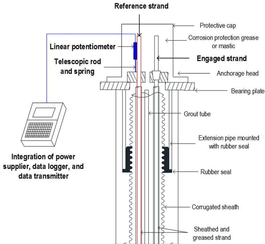
Fig. 4. Main components of the automated self-inspection device on the anchorage head.
