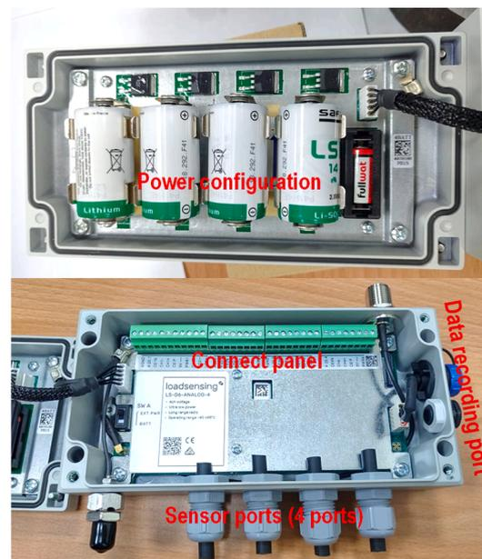
(b) Integration device (integrated with power supplier, data logger, data transmitter)
