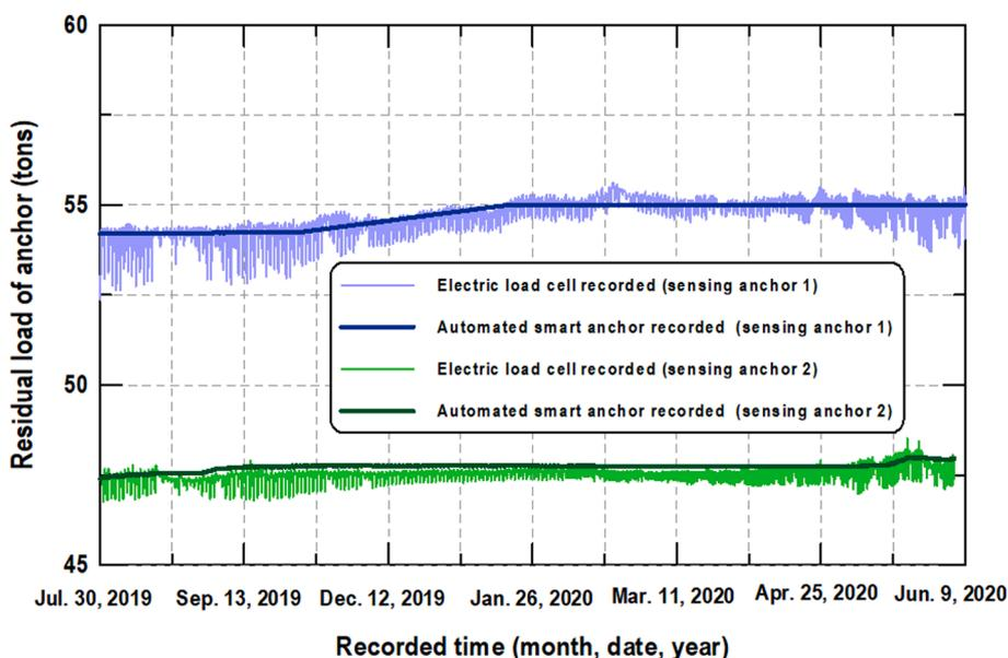
Fig. 10. Comparison of recorded data for the automated smart anchor and electric load cell from field sensing anchors 1 and 2.
