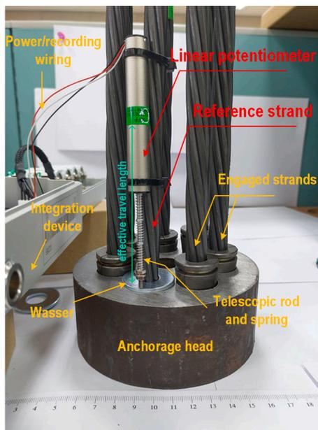
(a) Linear potentiometer mounted on reference strand
