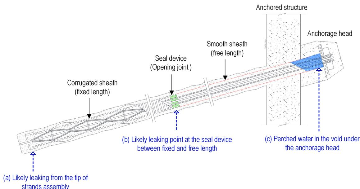
Fig. 1. Possible sources of water leakage into strands of conventional ground anchors in Taiwan.
