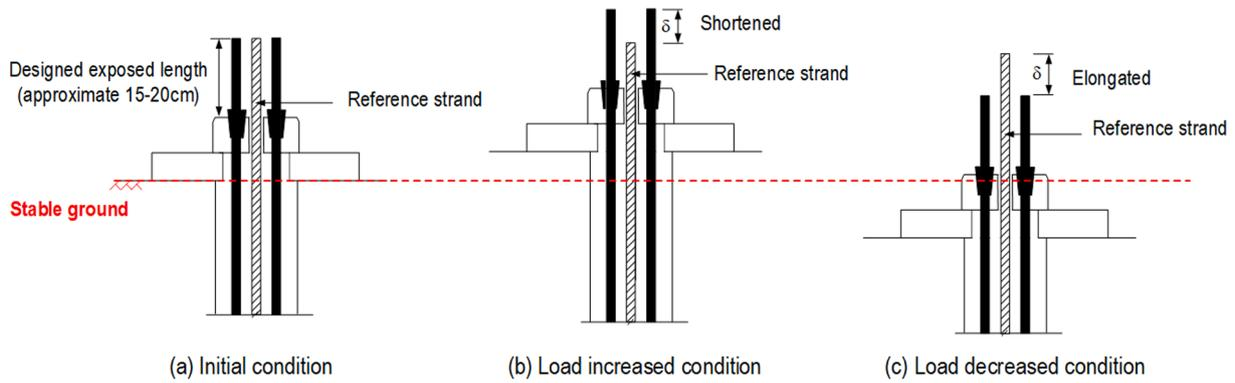
Fig. 3. Self-inspection for anchor load change of the smart anchor: (a) initial condition; (b) load-increased condition; (c) load-decreased condition.
