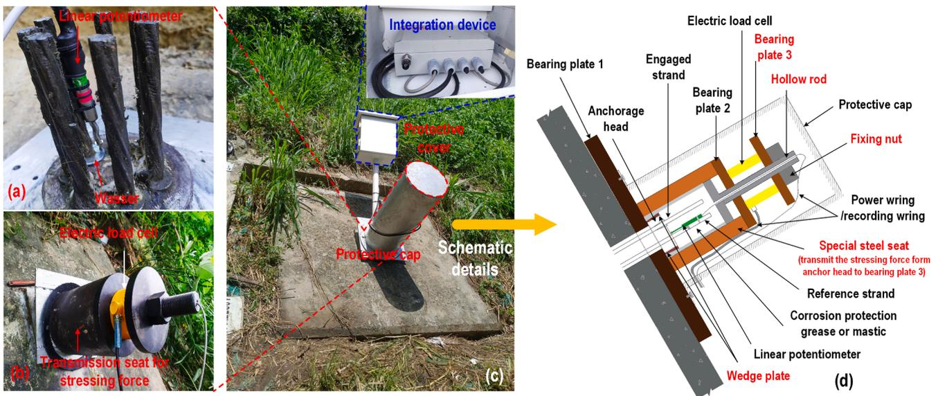
Fig. 9. Automated recording devices set up on the sensing anchors: (a) linear potentiometer mounted on the reference strand and washer placed on the wedge hole; (b) set up the special steel seat and electric load cell; (c) integrate device protected by the protective cover; (d) schematic of the automated devices in the protective cap.
