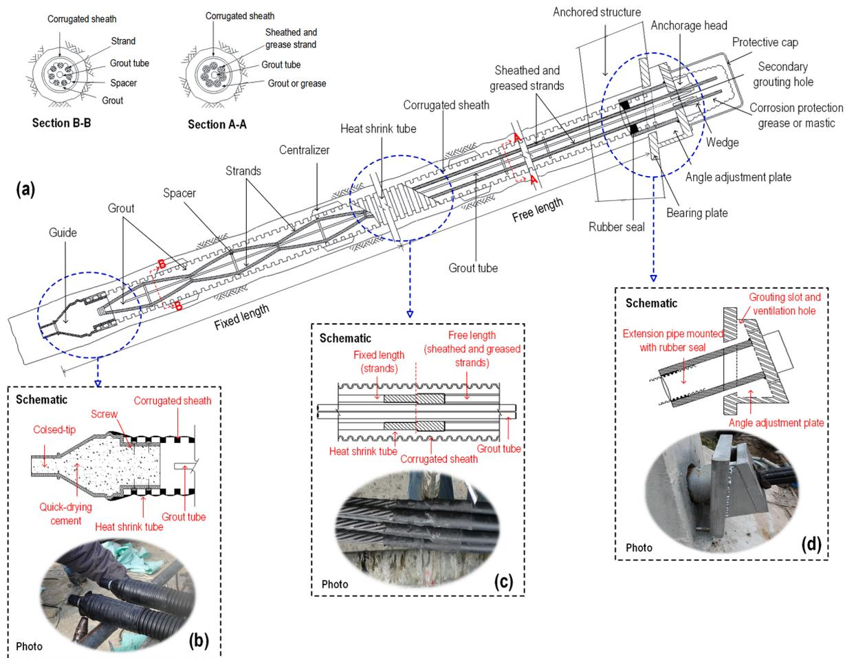
**Fig. 2.** Production of the smart anchor: (a) schematic of the fully corrosion-protected production; (b) details and photo of the closed-tip strand assembly; (c) details and photo of the opening joint removed; (d) details and photo of the custom bearing plate assembly under the anchorage head.
