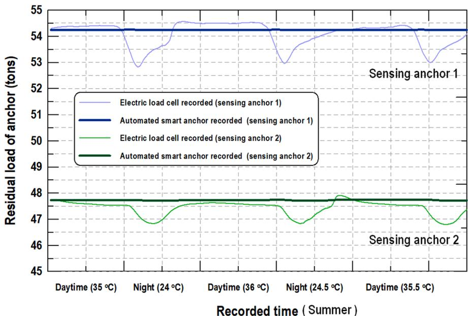
Fig. 11. Effect of environmental temperature on the recorded data for the automated smart anchor and the electric load cell.
