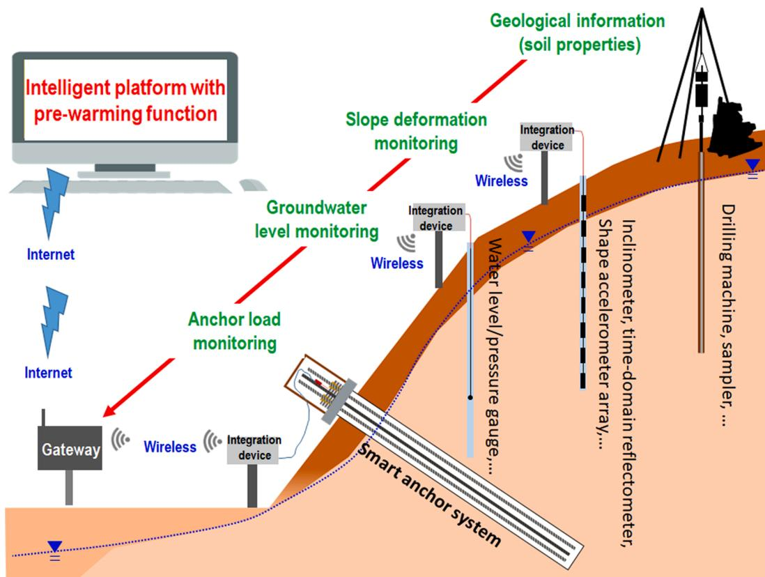
Fig. 13. Concept and future development of an intelligence platform for the smart anchor system.
