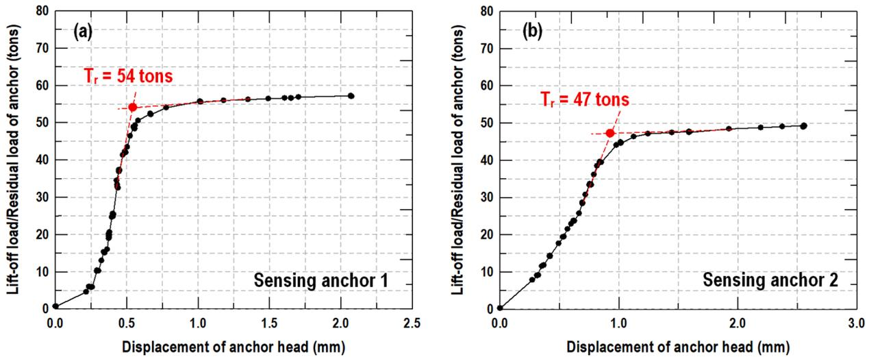
Fig. 8. Lift-off test result and residual load of: (a) sensing anchor 1 and (b) sensing anchor 2.
