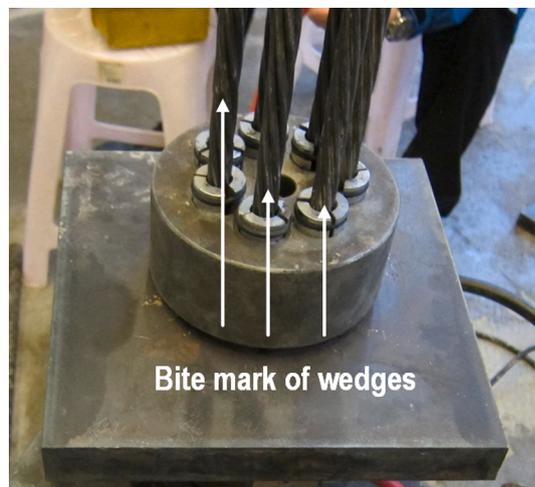
Fig. 14. Photo of a weak location and bite marks on the strand.
