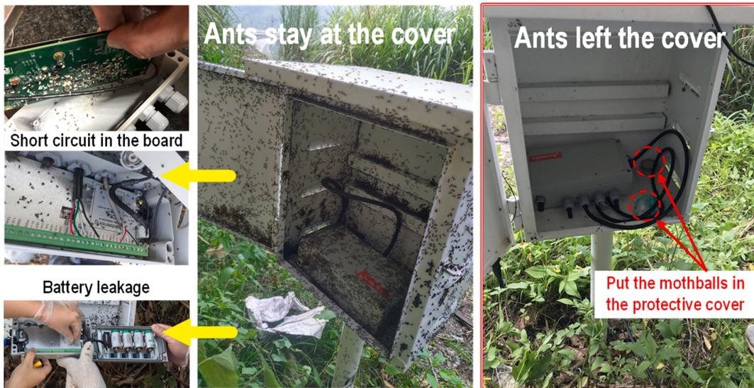
Fig. 12. Environmental impacts on the integrated device and damage prevention in the field.
