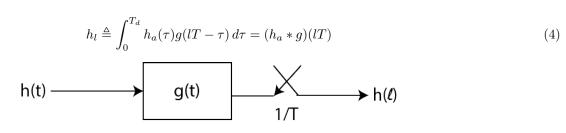
Hence, the equivalent digital filter  $\{h_l\}$  is just the convolution of  $h(\tau)$  and pulse  $g(\tau)$  sampled at rate  $\frac{1}{T}$ . The following figure is an L-"Tap" Channel, where L is the range of index l where  $h_l$  is nonzero.
