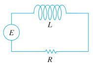
Consider the above LR circuit, where  $E(t) = 10 \sin(t)$  volts, R = 10 ohms, L = 0.5 henry, and initial current i(0) = 0. Find i(t).
