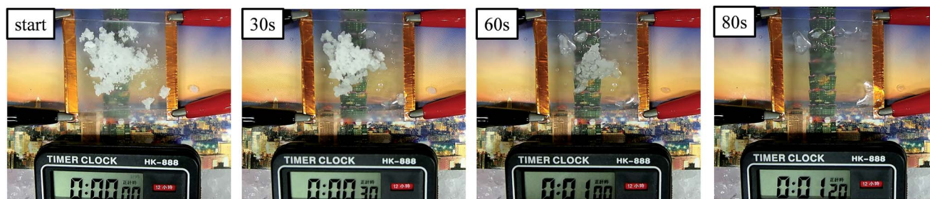
Fig. 8 Demonstrations of the snow-cleaning device based on AgNW-PI transparent electrode at the applied potential of 9 V (surrounding temperature: 5 °C).
