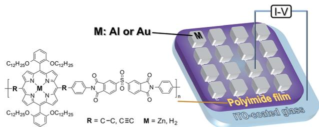
Fig. 1 Chemical structure of porphyrin-based PIs and memory device.
