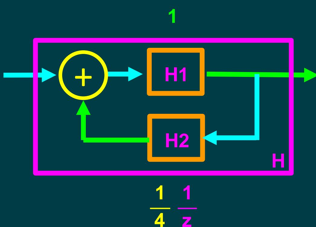
$$\begin{aligned} H &= \frac{H_1}{(1 - H_1 \cdot H_2)} \\ &= \frac{1}{(1 - 1 \cdot \frac{1}{4} \frac{1}{z})} \\ &= \frac{1}{(1 - \frac{1}{4} \frac{1}{z})} \end{aligned}$$
