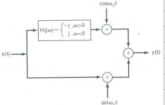
**8.25.** A commonly used system to maintain privacy in voice communication is a *speech scrambler*. As illustrated in Figure P8.25(a), the input to the system is a normal speech signal x(t) and the output is the scrambled version y(t). The signal y(t) is transmitted and then unscrambled at the receiver.
