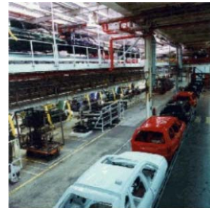
Final Assembly: Marriage of chassis and body
