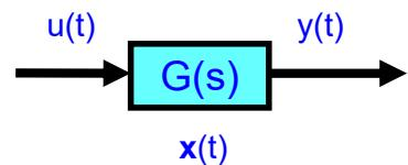
$$\begin{aligned}\frac{d}{dt}x(t) &= Ax(t) + Bu(t) \\ y(t) &= Cx(t) + Du(t)\end{aligned}$$
