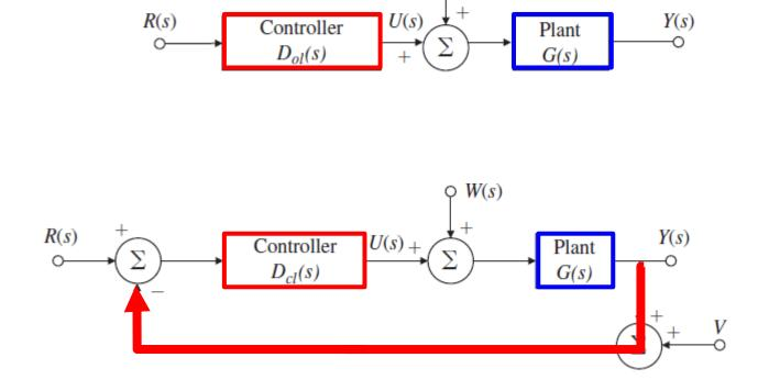
Closed-loop system showing reference, R, control, U, disturbance, W, output, Y, and sensor noise, V
