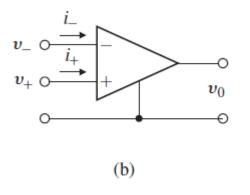
$v_{+} = 0$ Assume connected to ground,
