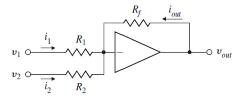
• From  $v_{+} - v_{-} = 0$ , we have  $v_{-} = 0$
