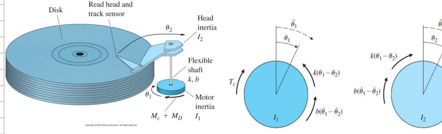
Model (Equations of Motion: Rotational motion)
