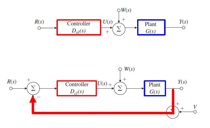
Closed-loop system showing reference, R, control, U, disturbance, W, output, Y, and sensor noise, V
