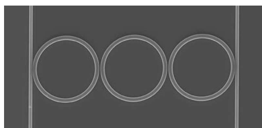
Fig. 7. SiN waveguide add/drop filter with a 50-dB extinction ratio demonstrated at MIT [31] (figure courtesy of E. Ippen).
