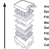
Anode core (+) Sponge pad Filter paper Membrane Gel Filter paper Sponge pad Cathode core (-)
