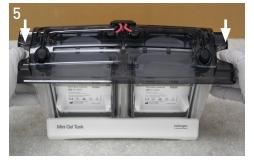
**5.** Make sure the power supply is **off**. Place the lid on the tank and plug the electrode cords into the power supply. Turn the power supply on to begin transfer.
