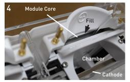
**4.** Add 1X transfer buffer to the module core if the sandwich is not completely submerged.
