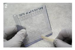
**2.** Remove the comb, and peel away the tape at the bottom of the gel cassette. Rinse the wells 3 times with 1X buffer.
