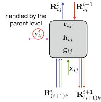
Fig. 8 Subsystem  $ij$  within ATC
