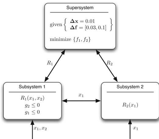
**Fig. 9** Bi-level structure of Eq. (7)
