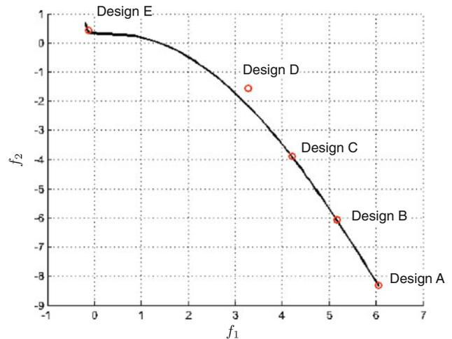
**Fig. 10** Design alternatives on the Pareto set using ATC
