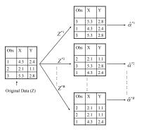
A graphical illustration of the bootstrap approach on a small sample containing n=3 observations. Each bootstrap data set contains n observations, sampled with replacement from the original data set. Each bootstrap data set is used to obtained an estimate of  $\alpha$ .
