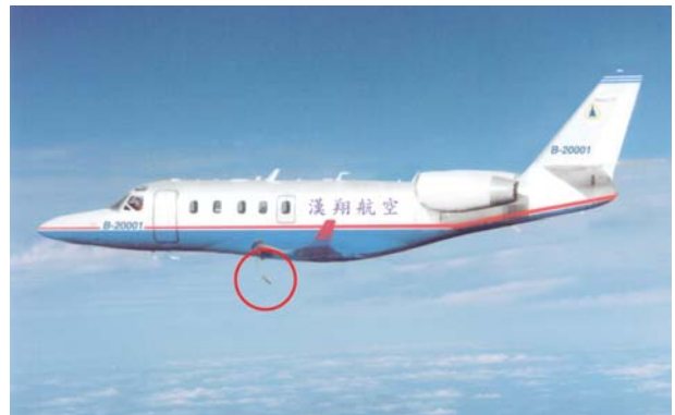
FIG. 1. The Astra SPX jet releasing a dropwindsonde (circled) during a test flight in March 2003.
